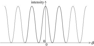
Award [3] for correct graph that shows modulation by single slit diffraction.
